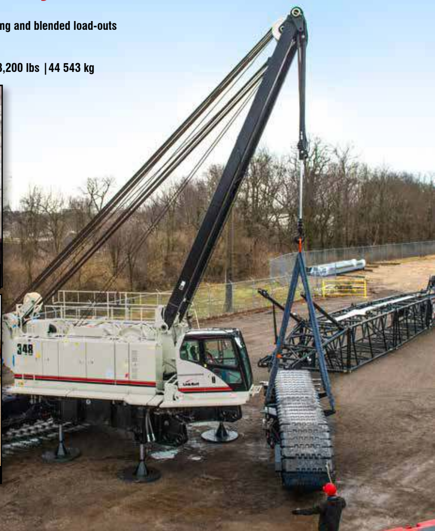
Complete counterweight removal/assembly from ground level
