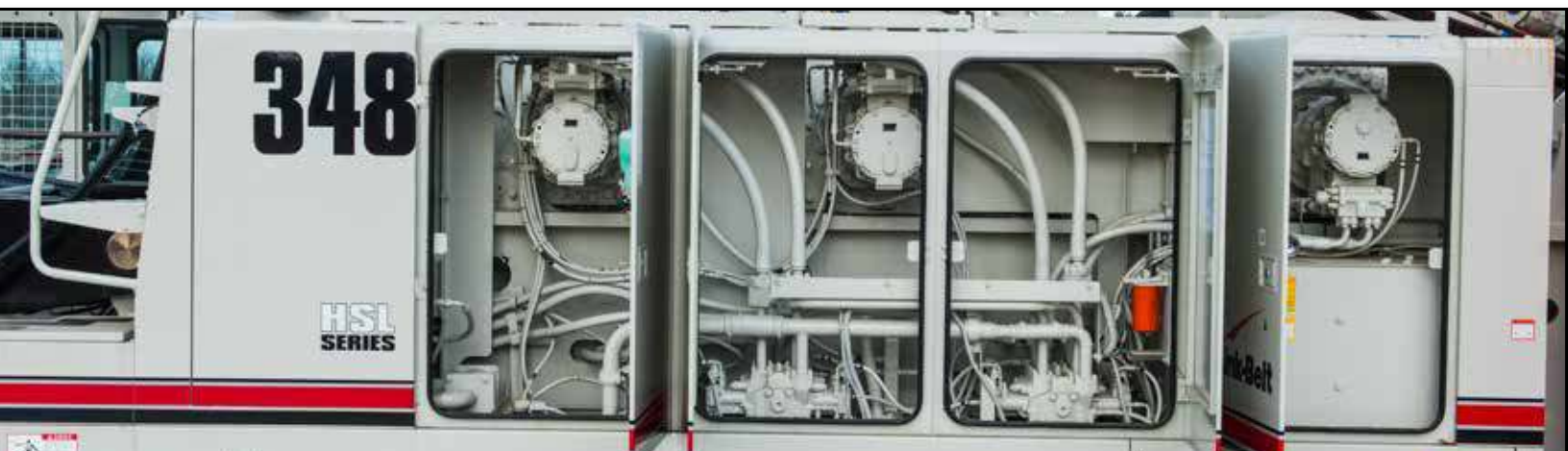
Excellent access for all routine engine and hydraulic maintenance
