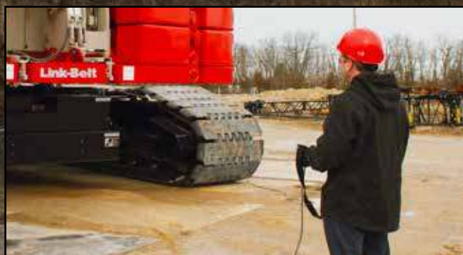
Complete counterweight removal/assembly from ground level
