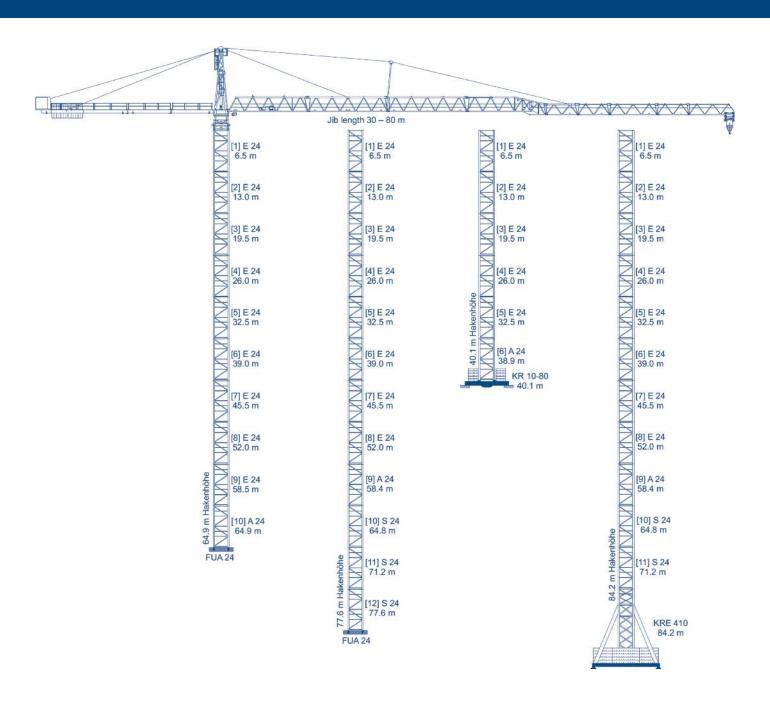
Tower combinations according to C 25 wind data.
