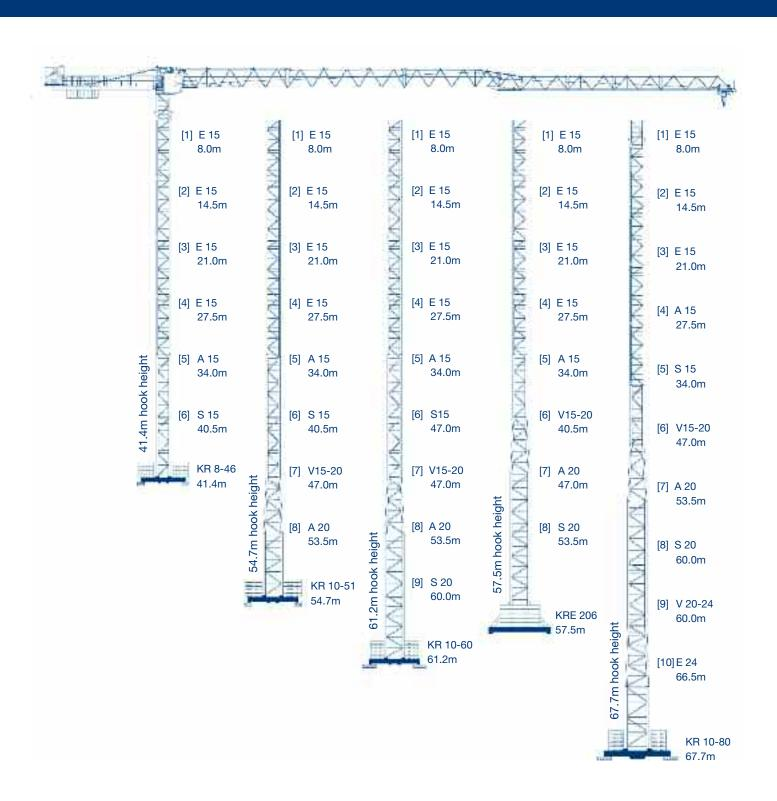
Tower combinations according to C 25 wind data.
