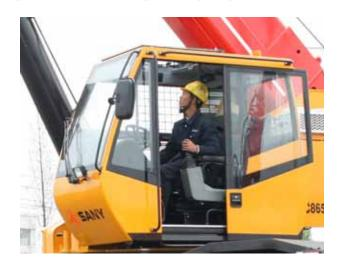
Spacious ergonomic cab with all steel construction. Optimum visibility, tinted safety glass throught. Opening skylight with visor and wiper system. Sliding door on the left hand side and a framed sliding window on the right hand side. Acoustical foam to absorb noise and insulate the cab. Deluxe six-way adjustable seat is equipped with mechanical suspension and includes arm rests and head rest.
