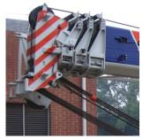
Formed boom made with high-yield steel which reduces the operating weight of the boom and maximizes performance.
