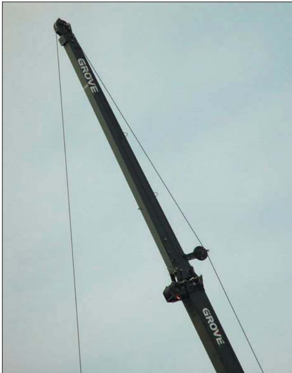
Max. tip height of 146 ft. (44.5 m) w/45 ft. (13.7 m) telescopic extension.
