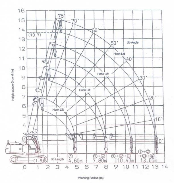
NOTE: The working ranges shown are determined with the machine under no-load condition, excluding jib deflection.
