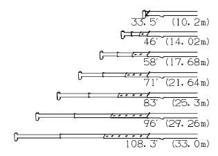
NOTE: Load radiuses for jib operation are given for reference with the boom fully extended to 108.3' (33m).
