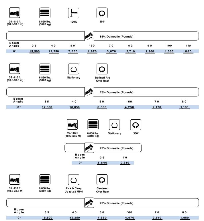
\*60 ft. boom length is with inner-mid extended and outer-mid & fly retracted
