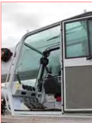
Spacious cab, adjustable seat, and conveniently located controls are common in all Tadano Mantis Cranes.
