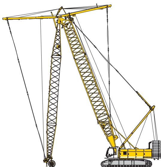
Erecting of main boom and luffing jib
